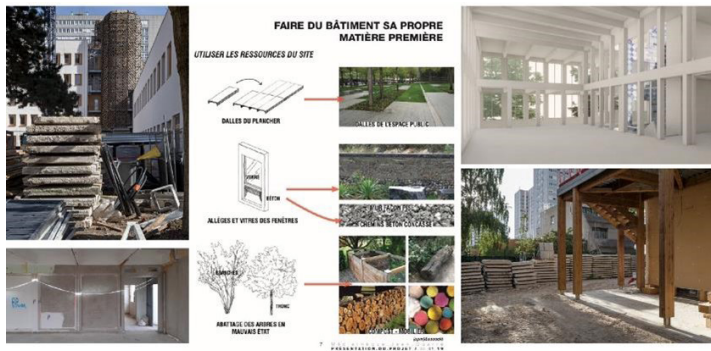
Figure 32. In-situ reuse of concrete floor slabs in the public space outside the Jean Quarré multimedia library
