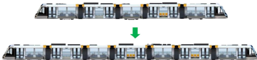
Figure 6: Extension of a Citadis 305 train to a Citadis 405.
